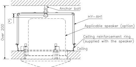
(\*) The exposed length of the anchor bolt on which the securing nut will be tightened must be no longer than 26 mm in order to prevent the bolt from contacting the speaker and thus interfering with correct installation.
