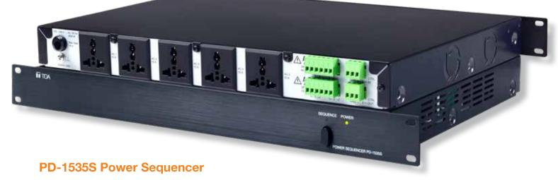
The TOA power sequencer helps to prevent AC power breakers tripping and protects your equipment from high power surges. Using a power sequencer to ensure proper equipment shutdown, you can prevent noise generated by front-end equipment and also prevent damaging your speakers. Designed with 5 AC outputs and 2 speaker zone, it has selectable delay of power on and off and can cascade up to 4 units. It is your ideal sequencing choice.
