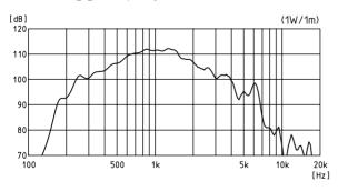
These high and low range frequency characteristics is one of the key issues to horn speaker sound quality. Particularly, we understand that optimised high range contributes greatly to improving the articulation of outdoor broadcasts. Attenuation in the air is more conspicuous for the high frequency ranges.
